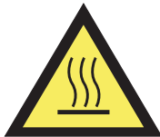
Fig. 6.14 Hot Surface Hazard Symbol
