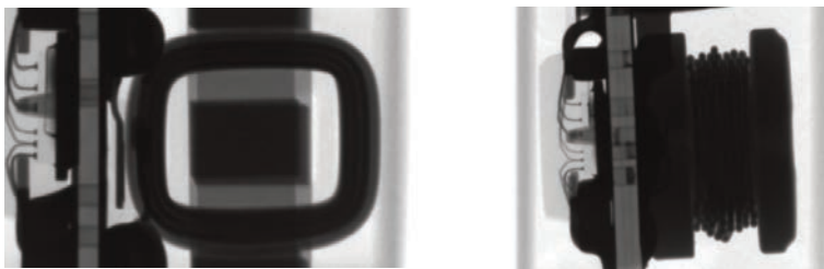
Fig 7.18: X-ray comparison between the shielded inductor used in RECOM's R-78 switching regulator (left image) and the unshielded inductor used in a competitor's copy product (right image).
